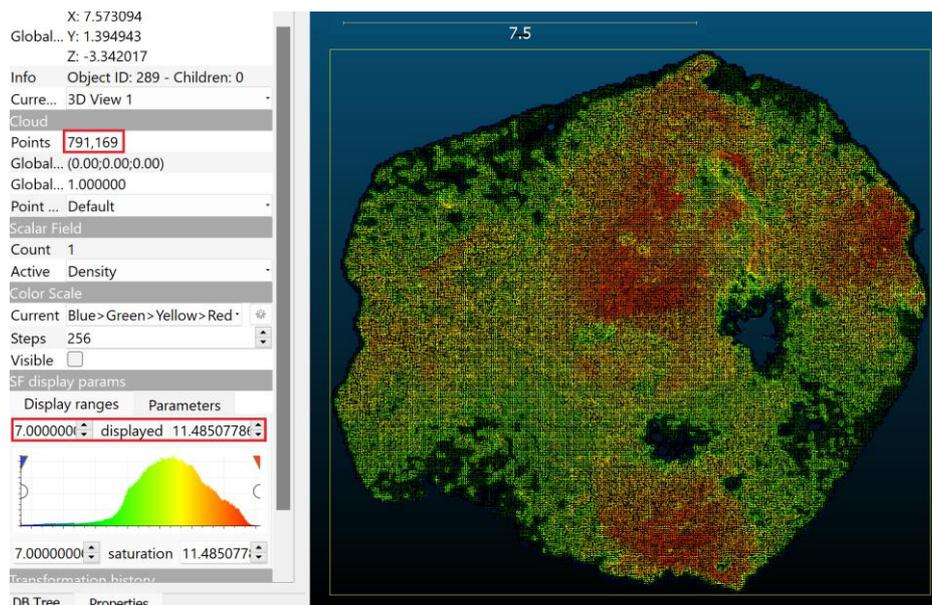
Fig. 7. The model filtered in CloudCompare by the set minimum and maximum density of the point cloud with a histogram and information about the number of points (screenshot from CloudCompare; own elaboration).
