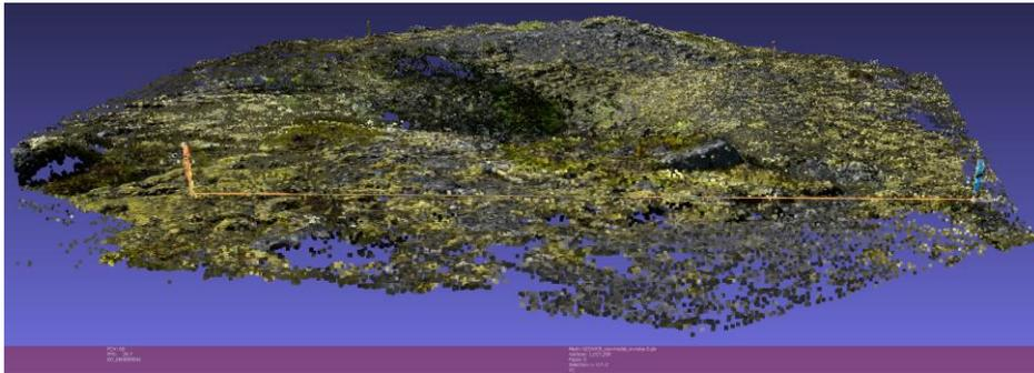
*Fig. 6. An example of a point cloud cleared of noise with visible stakes – measuring the distance between stakes on the model to calculate the scale factor (screenshot from MeshLab; own work).*
