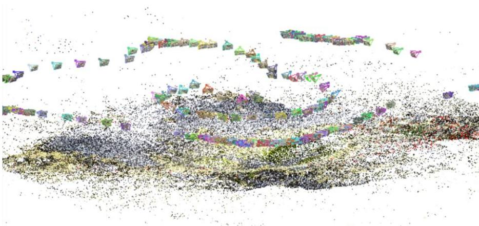
*Fig. 4. Arrangement of selected film frames along the route around an example of a kettle-hole against the background of a sparse point cloud of the model (screenshot from VisualSfM; own elaboration).*
