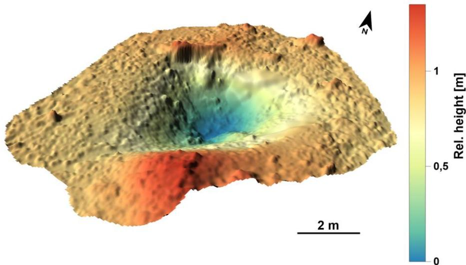
Fig. 9. An example of a DTM of a kettle-hole in a 3D view with a raster resolution of  $0.05\text{ m} \times 0.05\text{ m}$  with bottom relief reconstruction in the place of trees (own elaboration).
