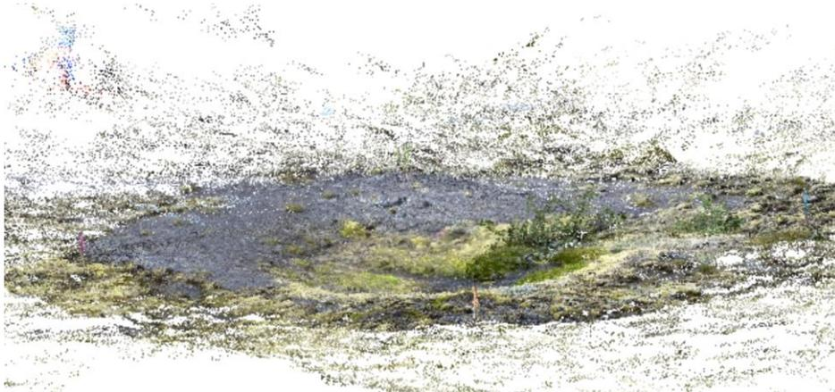
*Fig. 5. An example of a dense point cloud with noise obtained with the VisualSfM application and the PMVS/CMVS algorithm (screenshot from VisualSfM; own work).*
