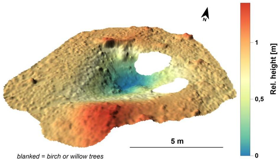
Fig. 8. An example of a DTM of a depression in a 3D view with a raster field resolution of  $0.05\text{ m} \times 0.05\text{ m}$  with fragments cut out due to birch colonisation (own elaboration).
