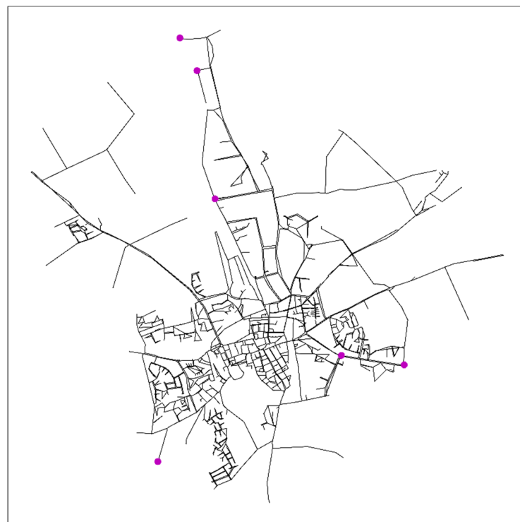
Figure 2. Illustration of the EPANET-model of the drinking water distribution network of City X. Connections to the utility's transport network (modeled as reservoirs in the hydraulic model) are indicated by a magenta circle.
