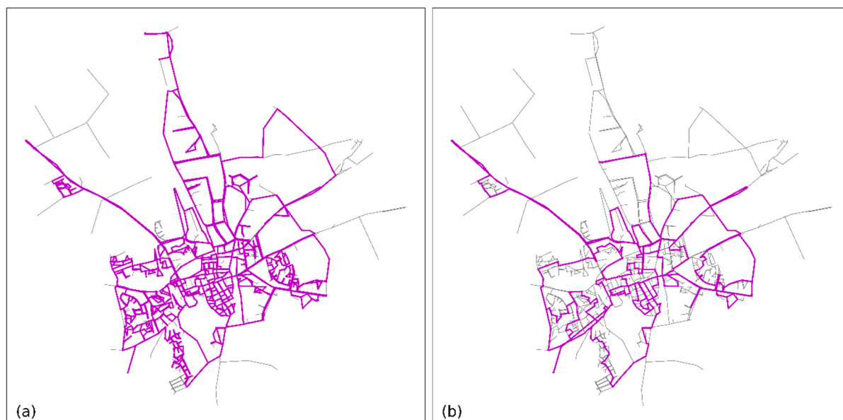
Figure 4. Layout of the secondary (magenta) and tertiary (grey) pipes in the current design (a) and the optimized design (b). Compared to the current design, the optimized design shows a clearer secondary structure and a greater number of branched tertiary pipes.
