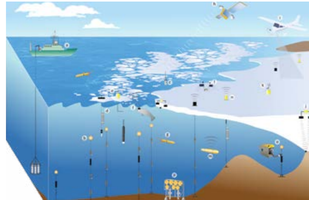
The schematic above shows an integrated system of under-ice observational platforms required to determine the contribution of oceanic heat to ice shelf melt. These include ship-based observations (a); moored instrumentation (b); ice-capable profiling floats (c); ice-tethered profilers (d); ice-mass buoys (e); seal tags (f); gliders (g); radars (h); automatic weather stations (i); GPS, boreholes and other landers (j); sensors/moorings deployed through boreholes (k); moorings deployed by remotely operated vehicles (l); bottom landers (m) (Newman et al., 2019, Figure 7, Frontiers in Marine Science ).
