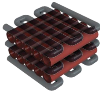
Fig. 4: Schematic depiction of a possible cultured-meat scaffold design. The Red tubes represent perfusable channels enclosed with muscle fibers, layered on top of each other in parallel with interstitial layers of adipose and fibroblast cells
