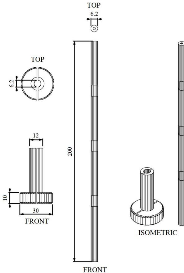
**Fig. 10.** Schematic of the 3-D printed OFS holder (unit: mm), from multiple views. Two distinct components are shown: 1) the component that slots into the Markus Chamber holder and 2) the cylindrical “guide tube” that is delivered through 1) and constrains the position of the sensor in a parallel orientation. Note: central channel of 2) is matched in diameter to that of the BT needle that holds the sensor.
