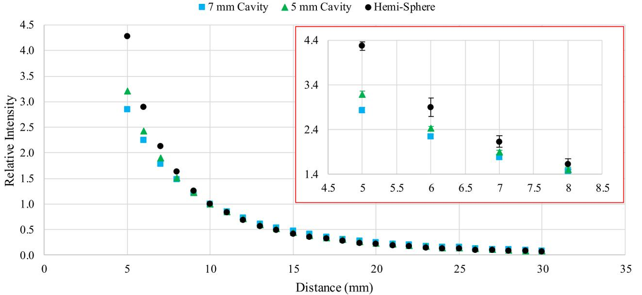
Fig. 4. Relative comparison of the fall-off in PCR along the transverse axis as a function of distance from the source, for each of the scintillator geometries considered in this work (normalized at 10 mm). An inset of the data from 5 to 8 mm is included on the right-hand side of the graph, rescaled for clarity.
