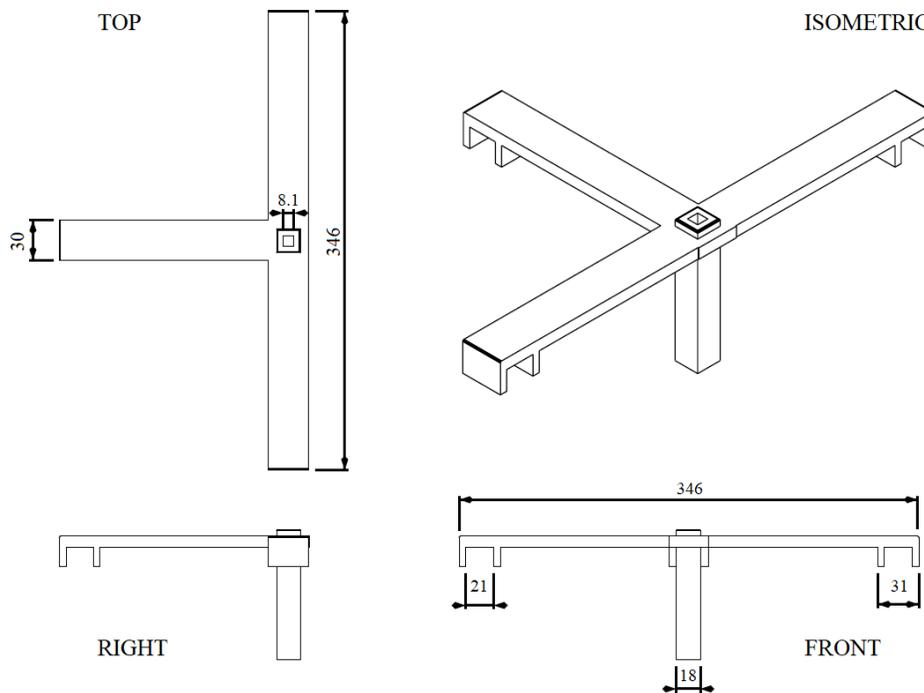
Fig. 8. Schematic of the 3-D printed T-junction top support for the source holder (unit: mm), from multiple views.
