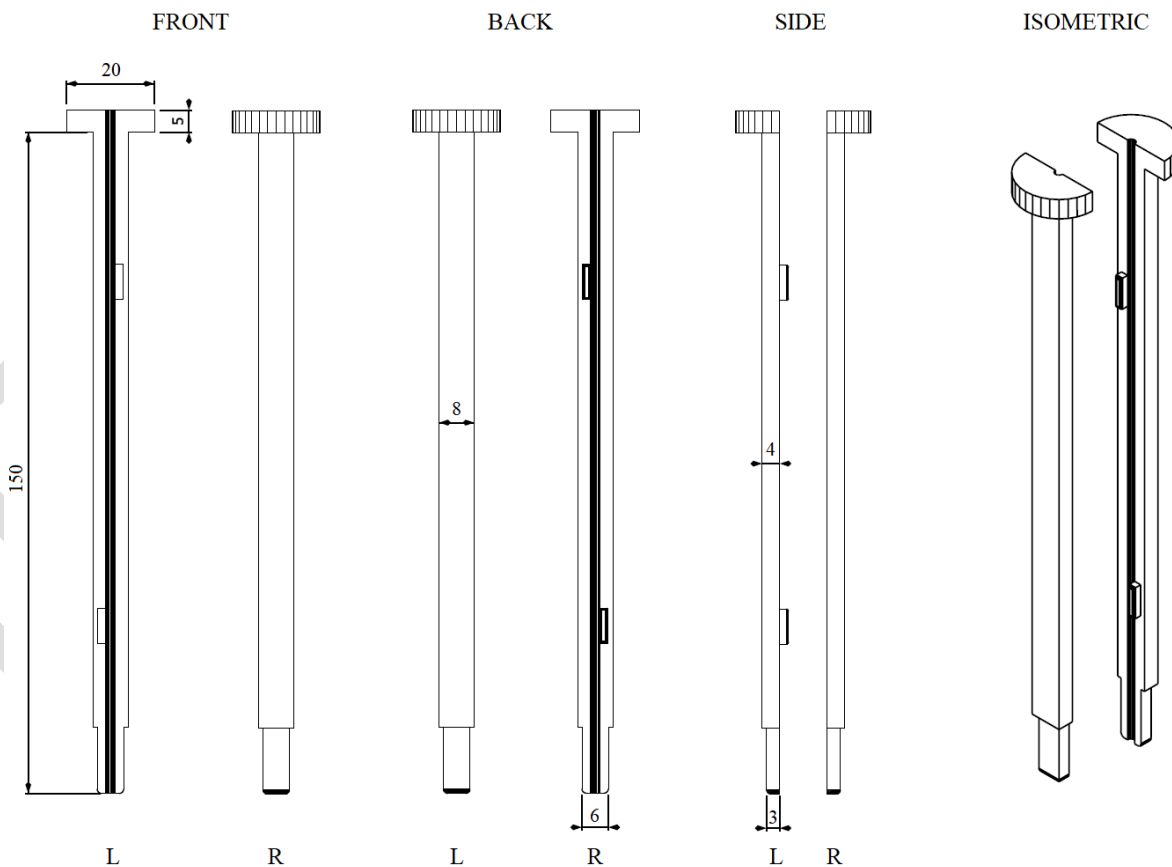
Fig. 9. Schematic of the 3-D printed source holder (unit: mm), from multiple views. This component is printed in two parts, left (L) and right (R). The central channel is matched in diameter to that of the BT needle that holds the source.
