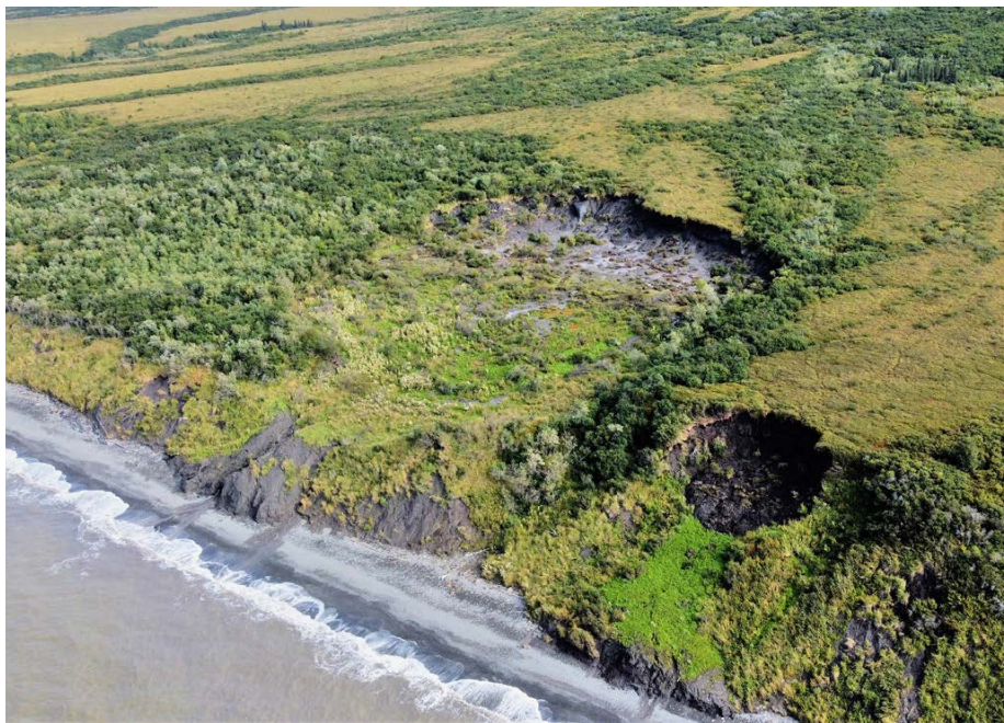
FIGURE 5. Thawing permafrost resulted in a large, older sinkhole (left, with vegetation growth inside) and a new sinkhole (right, with dark soil) on the coast six miles from Unalakleet. Photo credit: Ikaagun Engagement
