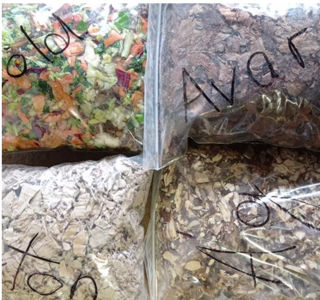
Figure 3: Samples of chopped biowaste analysed, from top left clockwise: i) mixed vegetable waste, ii) fallen leaves, iii) cardboard and iv) branches
