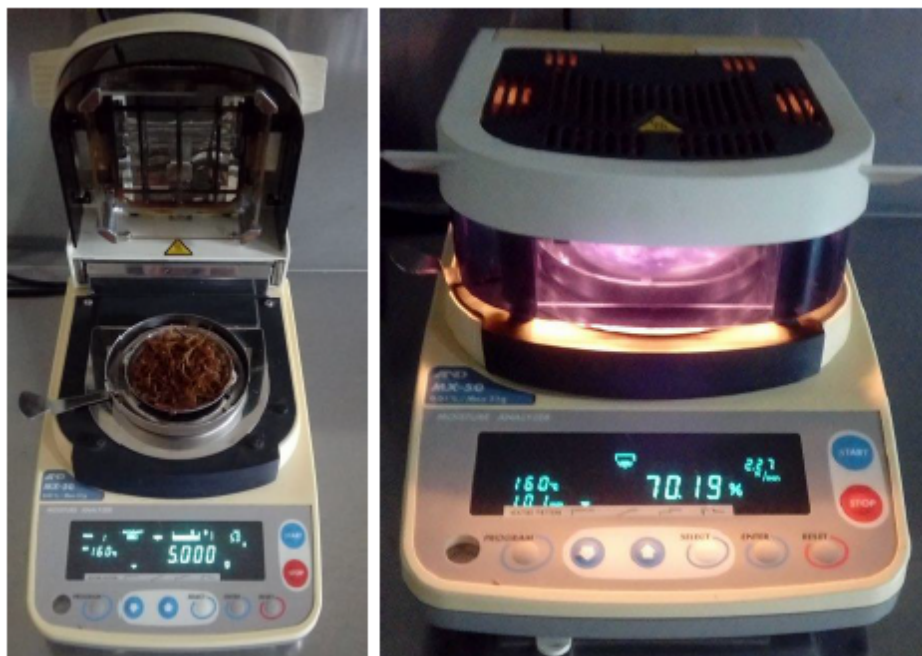
Figure 5: AND-MX-50 device for moisture content determination
