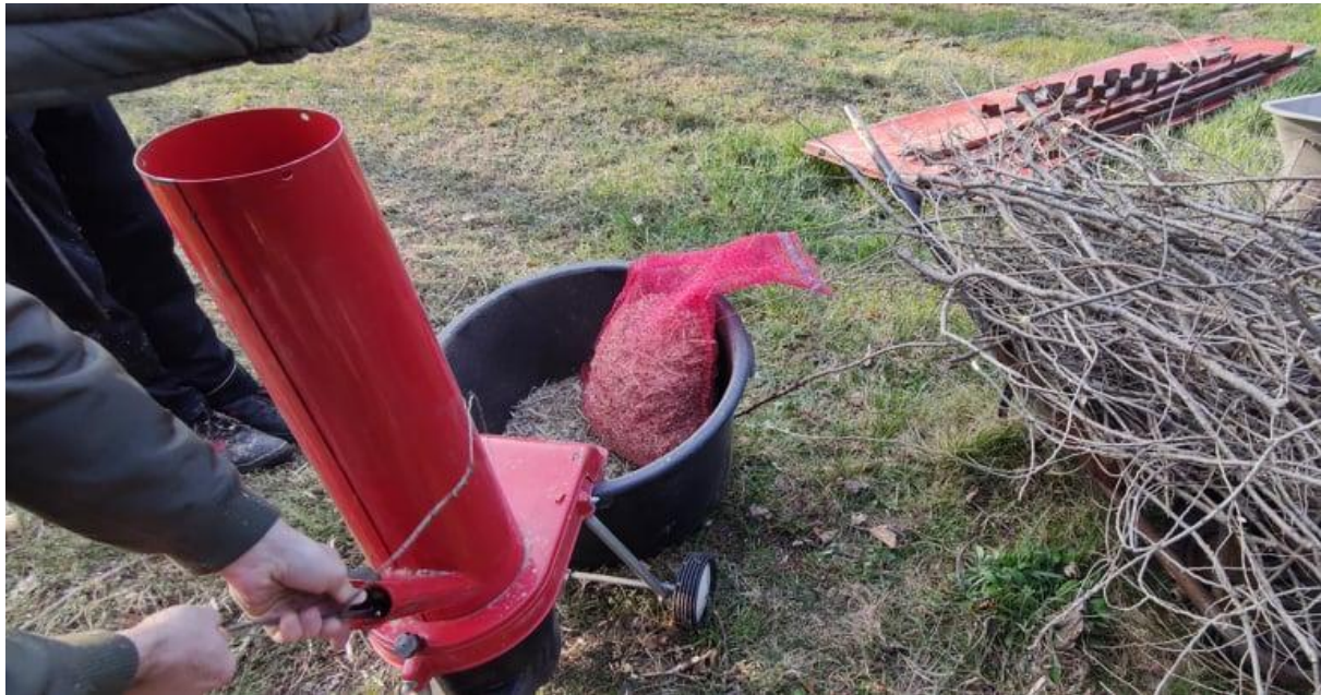
Figure 4: Chopping of the samples (branches on the figure) and storing the chopped samples in net bags
