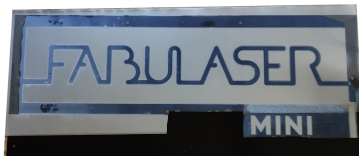
Figure 12: Example of post processing steps; the logo is applied to the Front Panel
