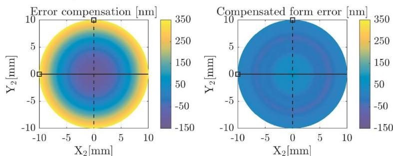
Figure 2: (a) Initial form error before the correction machining. (b) Reduced form error after the correction machining.
