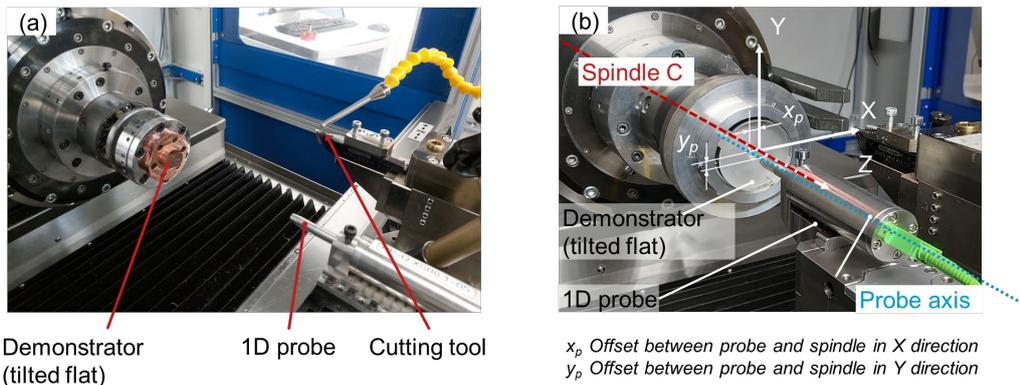
Figure 1: (a) The on-machine metrology system, integrated on an ultra-precision turning machine. (b) The probe offsets in X and Y direction with respect to the machine tool coordinate system.
