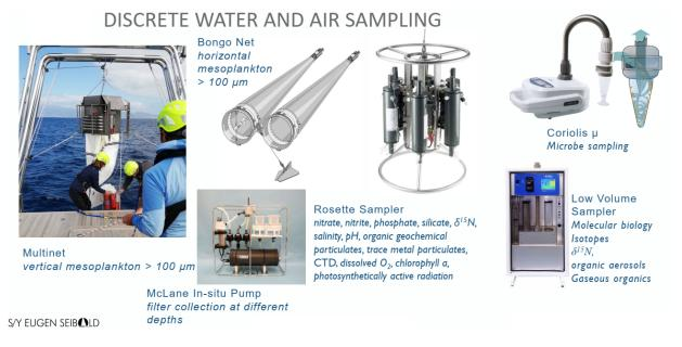
Figure 13. Eugen Seibold instrumentation for discrete water air sampling at selected stations
