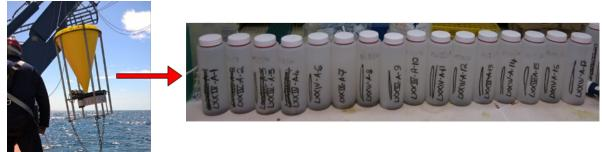
Figure 20. Left: Sediment trap being deployed; right: time-series of sediment trap samples collected at the SOG site.
