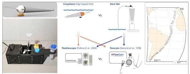
Figure 17. Coryphaena net and PlanktoScope v2.5 (left) and summary of tests performed on board SV Tara (right)
