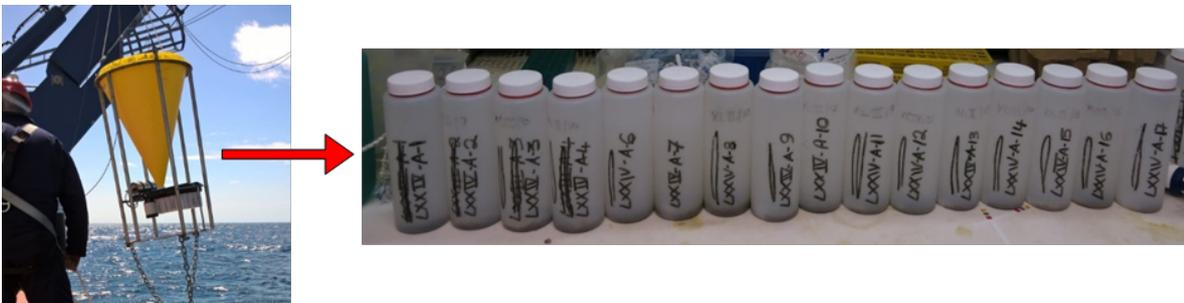
Figure 20. Left: Sediment trap being deployed; right: time-series of sediment trap samples collected at the SOG site.
