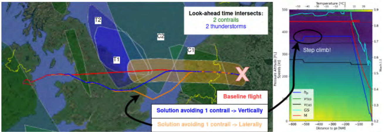
Fig. 9. Alternative trajectories for flight UAE161 (B777-300ER) from OMDB to EIDW (July 27, 2018)
