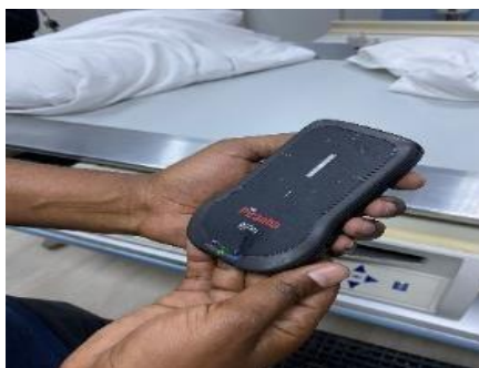
Figure 2: Show the recommended equipment for performing accuracy of reproducibility of exposure time and other tests: Piranha dosimetry MULTI X-ray meter of (Ocean Next™ software) Standard for Complies with relevant parts of the standards IEC 61674 and IEC 61676 for Dosimetry instruments. Such meter was used for the QC measurements
