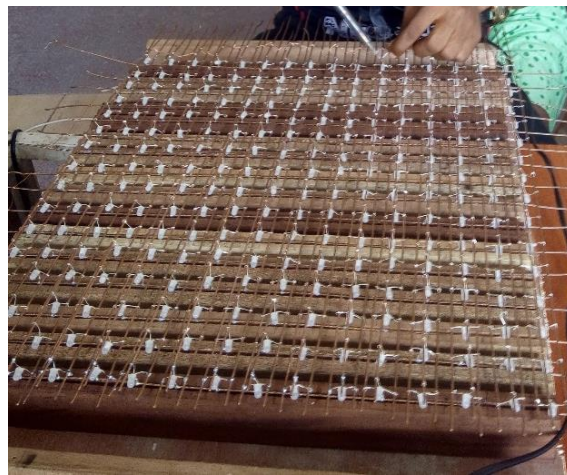
Figure 4. A single layer/slice of the LED cube
