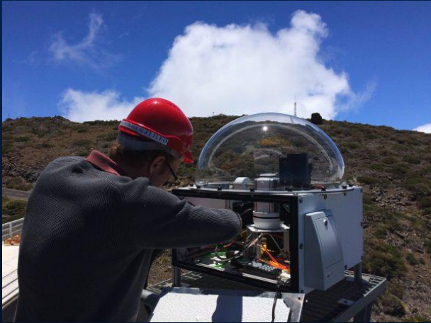
Installing the solar telescope at the TNG
