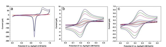
Figure 5. a) Electrochemical characterization of the structural stability and electrical independency of the coaxial electrodes for the inner (red), outer (dark blue) and short-circuited (light blue) electrodes recorded in 0.5 M sulfuric acid at 100 mV s<sup>-1</sup>; b,c) Cyclic voltammograms of the outer and inner electrodes in 1 mM ferrocene methanol in 0.1 M KNO<sub>3</sub> recorded at 5, 10, 25, 100, 150 and 200 mV s<sup>-1</sup>, respectively.
