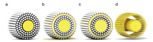
Figure 2. Scheme illustrating the elaboration steps of a miniaturized coaxial macroporous twin electrode. a) Gold microwire (250 µm) covered with a predefined number of 1 µm silica particle layers. b) Electrodeposition of the gold-nickel-gold layer through the colloidal silica template. c) Structure obtained after the selective dissolution of the nickel layer. d) Final electrode structure obtained after the dissolution of the silica template.
