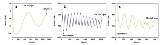
Figure 3. Examples of chronoamperometric curves recorded during the electrodeposition of a) the inner gold, b) the intermediate nickel, and c) the outer gold layers throughout the colloidal silica template.
