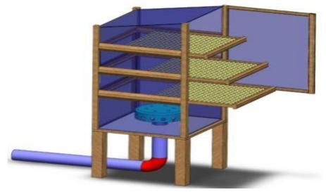
Fig. 1. b. Scheme of a greenhouse-type dryer
