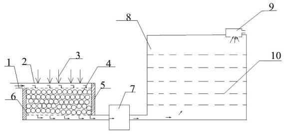
Fig. 3. Black agate home type solar air heater with solar dryer. here :
