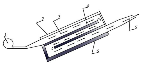
Fig. 2(a), Solar air collector with thermal storage material (a) below the absorber. here :
