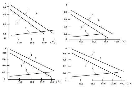
Fig.4. Dependences of the thermal efficiency of drying chambers "theoretical" "real" (2), as well as its decrease  $\Delta \eta_k$  (3) on the temperature of the drying agent at the outlet of it (t<sub>2</sub>) respectively at  $t_{1,\circ}C: t_1 = a - 70^\circ$ ; b-80°; at-90°; and g-100°C.
