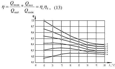
Fig.1. Dependence of the efficiency of the drying plant on the heating temperature of the drying agent in the solar collector  $*(t_1)$  and at the outlet of the drying chamber  $*(t_2)$ : 1, 2, 3, 4, 5 and 6 - respectively at\*  $t_2$ =75; 80; 85; 90; 95 and 100°C.
