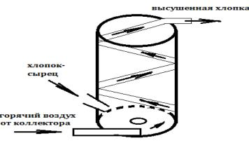
Fig. 1. Schematic diagram of a vertical dryer.
