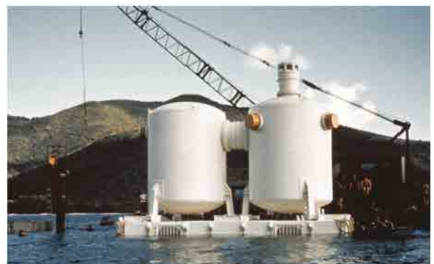
Tektite I. The laboratory was built in 1969 and submerged 15m in the waters off the Virgin Islands. Source: https://exploration.marinersmuseum.org/watercraft/tektite . Public domain.
