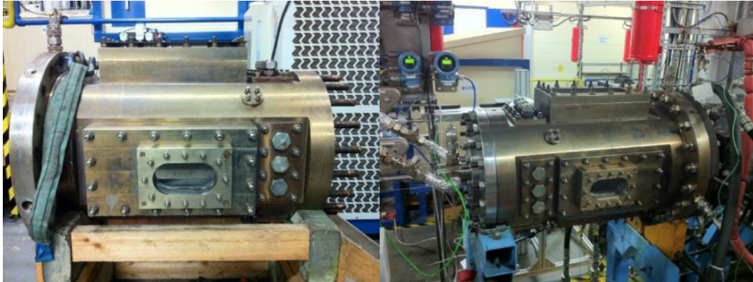
Figure 1: Photographs of HPOC during maintenance (left) and installed in the HPCR (right)
