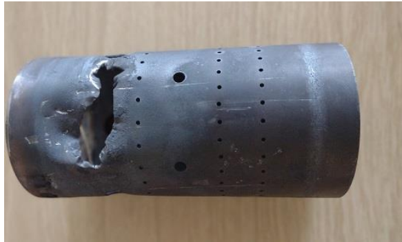
Figure 3: Combustor Can damaged during RQL 1 Test
