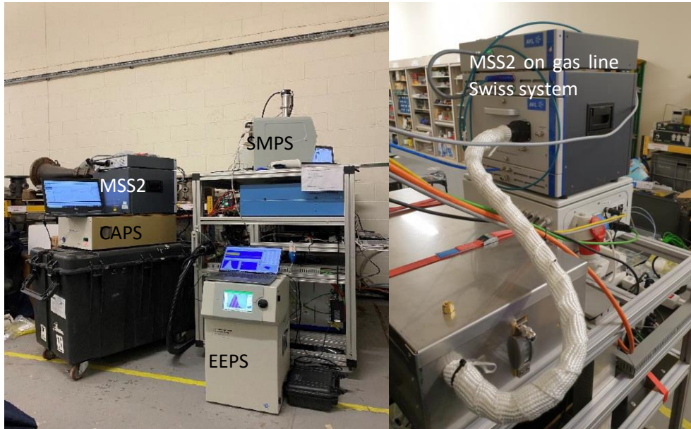
Figure 6 (a&b): Photographs of the Swiss system with the MSS2 on the nvPM line and the MSS2 on the raw line (during RQL 2) respectively
