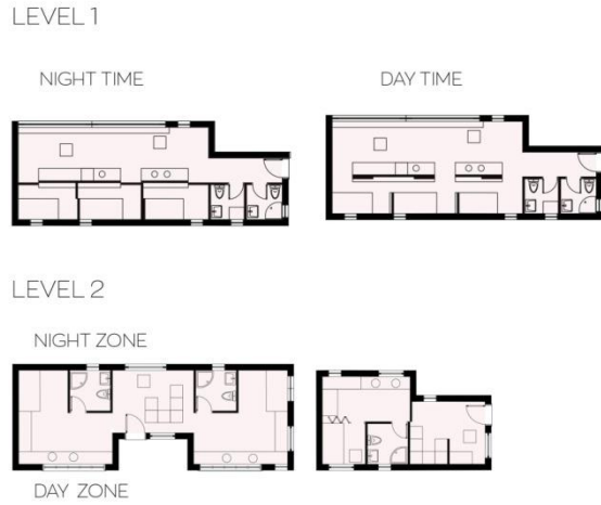
Photo 7: Night and day zones in level 1 and level 2
