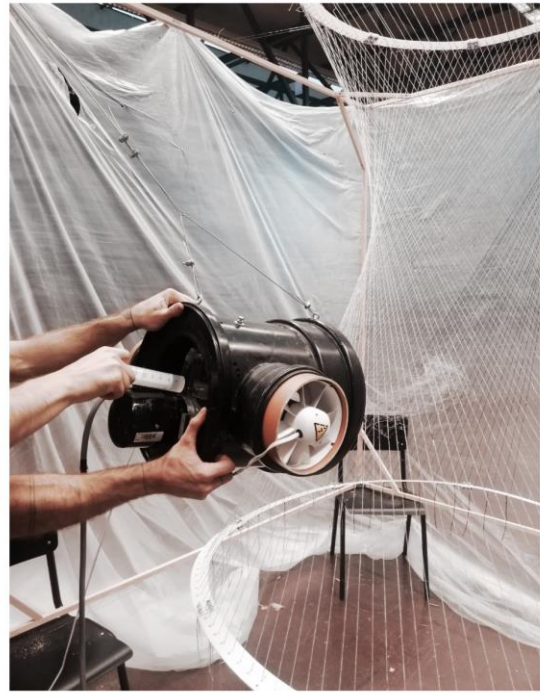
Figure 8. Application of nanofibre layer by centrifugal spinneret (nanofibre centrifuge) (right)
