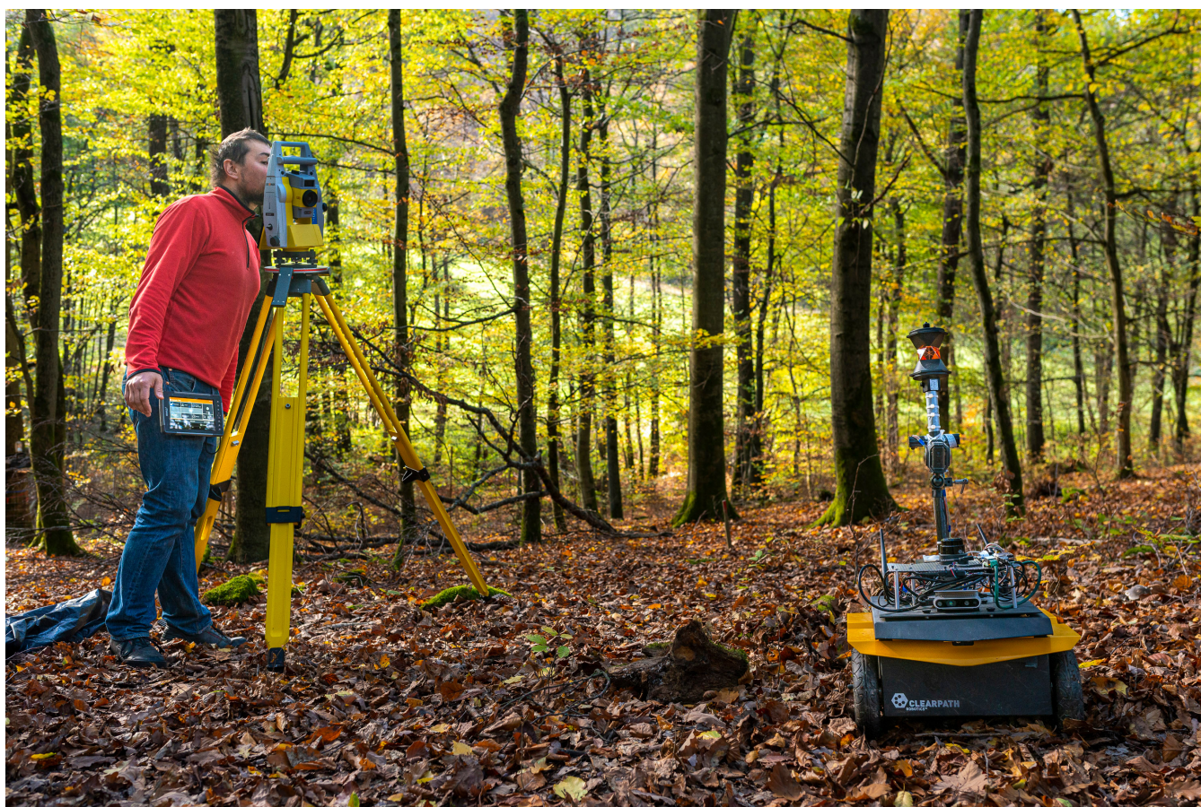
Figure 8. Setting-up for automatic measurements: Aiming the oriented robotic total station at the rover's prism.
