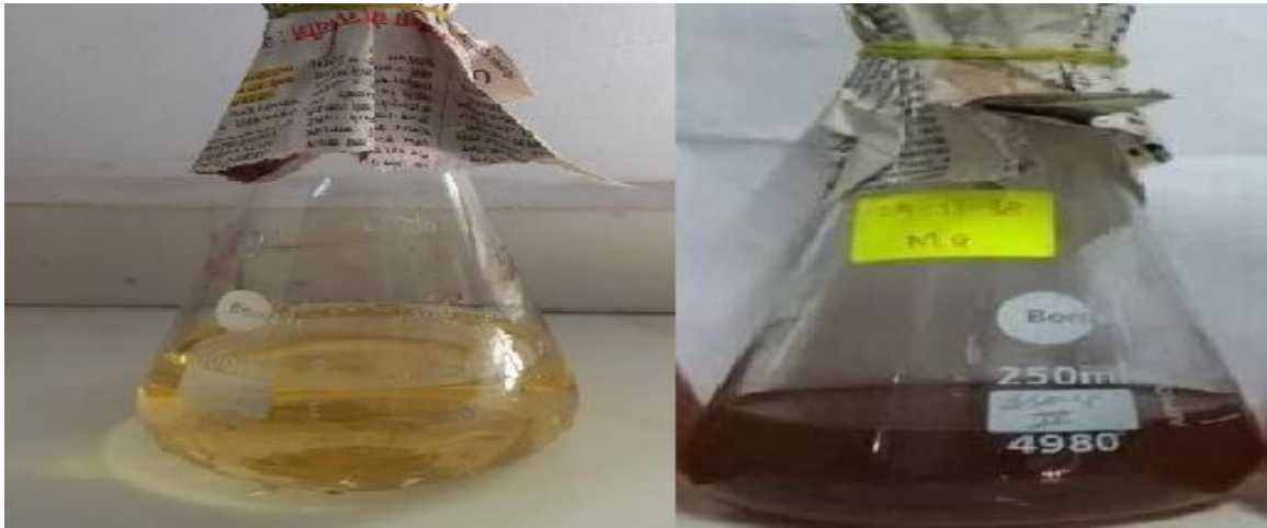
Photos 2: Formation of silver nanoparticles was detected by color change from Pale yellow to dark brown.
