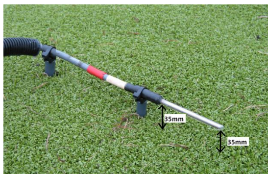
Figure 6. Grass minimum thermometer over an artificial surface
