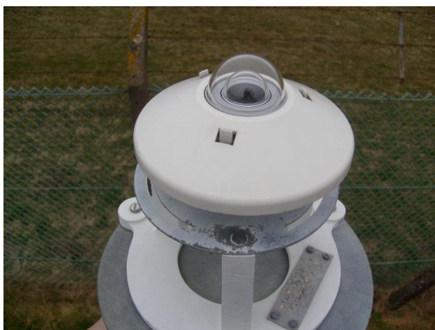
Figure 16. Pyranometer for measuring global radiation
