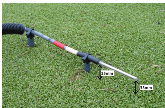
Figure 6. Grass minimum thermometer over an artificial surface
