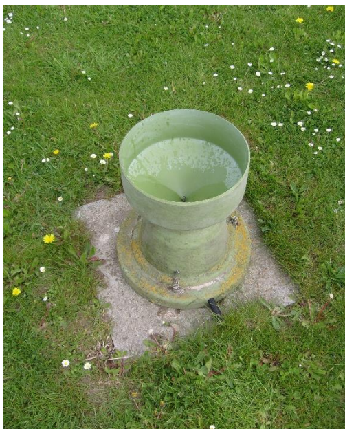
Figure 14: Tipping bucket raingauge
