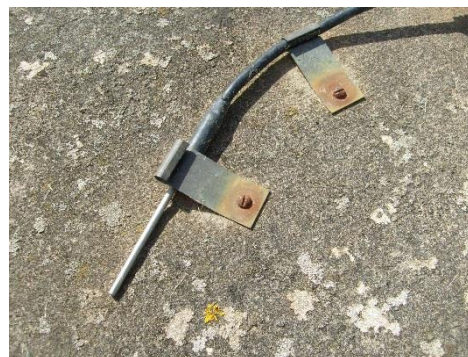
Figure 7. Concrete minimum grass thermometer
