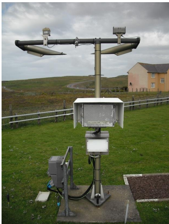
Figure 21. Present weather sensor
