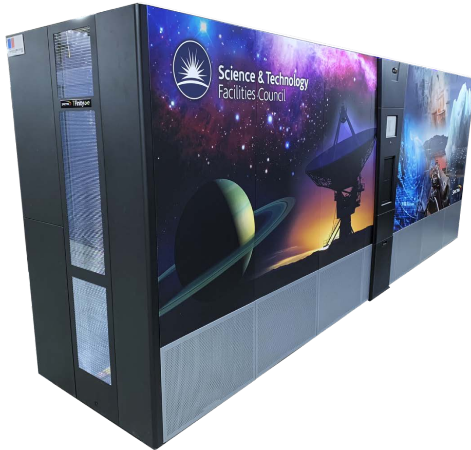
Figure 21: The Spectra Tape library which was procured and installed as part of the JASMIN Phase 5 upgrade.
