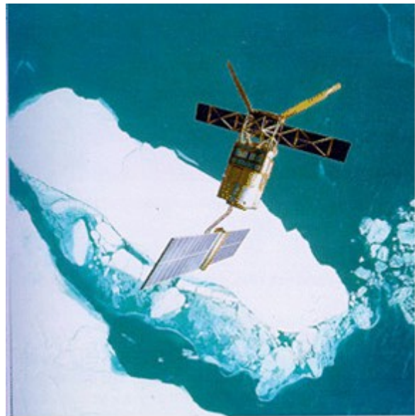
Figure 23. ATSR instrument collecting data on board the ERS 1 satellite
