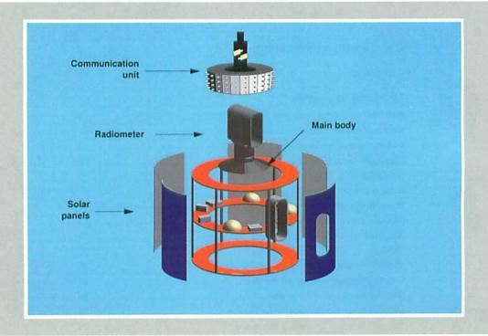
The Meteosat satellites are composed of a main cylindrical body to which six solar panels and a telecommunications payload (top) are attached. The radiometer, which generates the images, is located inside the cylinder together with most of the electrical systems and spherical tanks filled with propellant for the thrusters to perform attitude manoeuvres.
