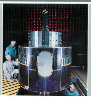
Meteosat barely resembles a "typical" satellite, reflecting the fact that its principal mission differs from that of most other satellites in geostationary orbit which are mainly concerned with telecommunications services. The main feature of Meteosat is a big cylinder containing a special telescope - the radiometer. This cylinder's shining dark blue cover consists of solar cells, and the two smaller cylinders stacked on top of it carry a telecommunications system and special antennas.
