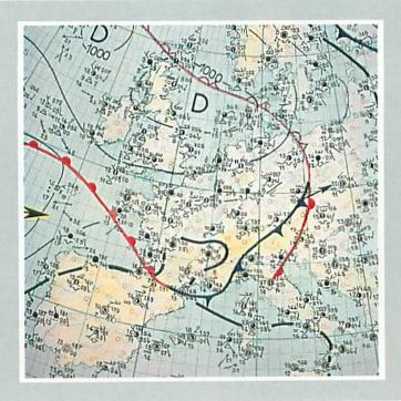
Weather can be described by many parameters: temperature, humidity, wind speed and direction, and above all barometric pressure. These and other data are measured twice a day by thousands of radiosondes released into the upper atmosphere by means of helium-filled balloons. This information is complemented by data from meteorological stations and satellites in polar and geostationary orbit.
