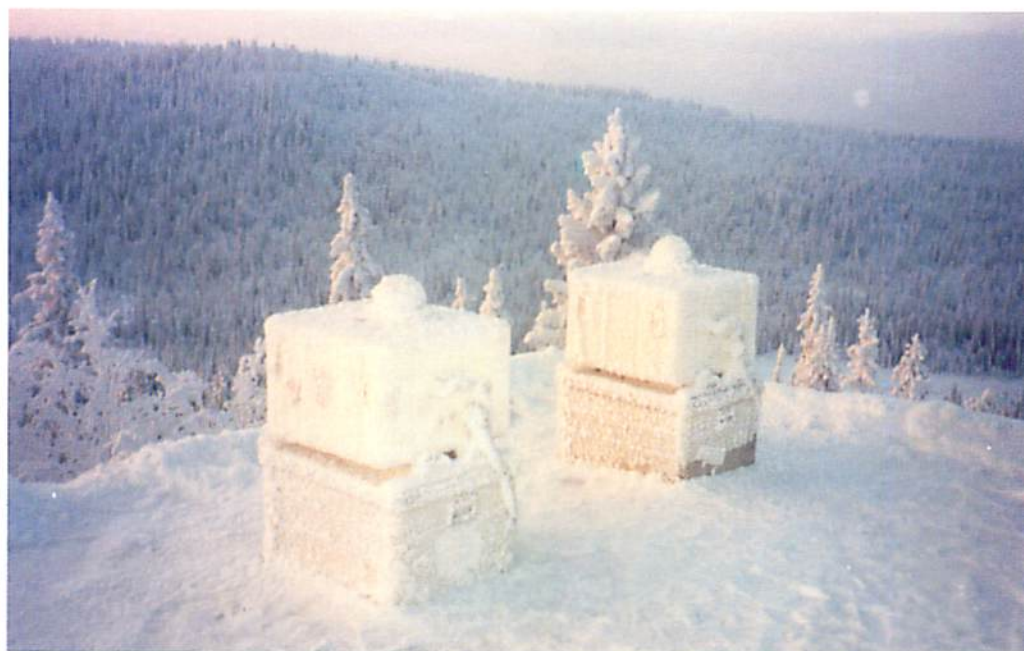
UV-visible spectrometers are widely in use for the monitoring of ozone, nitrogen dioxide, chlorine dioxide and PSCs. Because the measurements are performed in the visible during twilight, they are able to provide daily data, up to the latitude of the polar circle in winter, in all weather conditions, when more traditional UV instruments are blind. The picture shows two automatic SAOZ spectrometers developed at CNRS, under parallel testing in extreme conditions at ESRANGE, Kiruna, Sweden, in winter.
