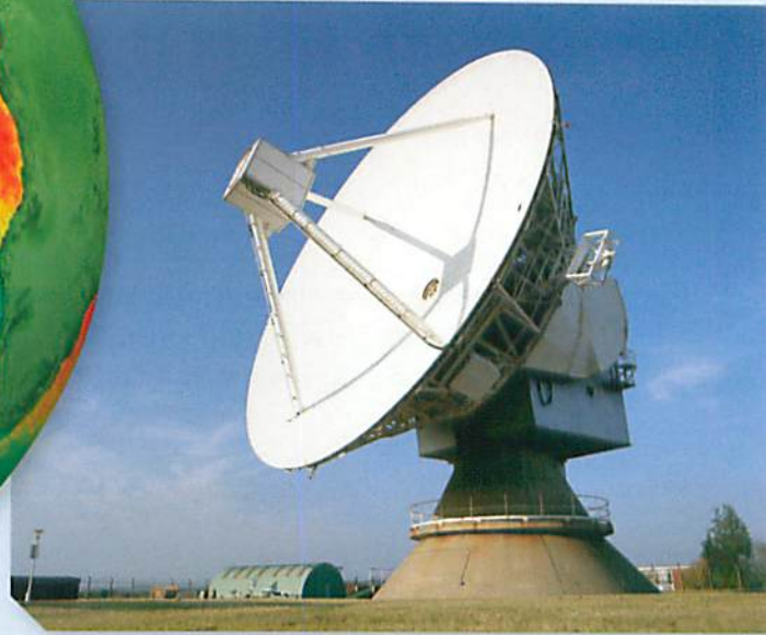
The Chilbolton Observatory in Hampshire helps atmospheric scientists research how rain develops to improve estimates of rainfall. The radar can distinguish rain from snow and ice, as well as the size of individual raindrops. A new radar allows scientists to see how and where convective clouds form and develop into rain clouds.
