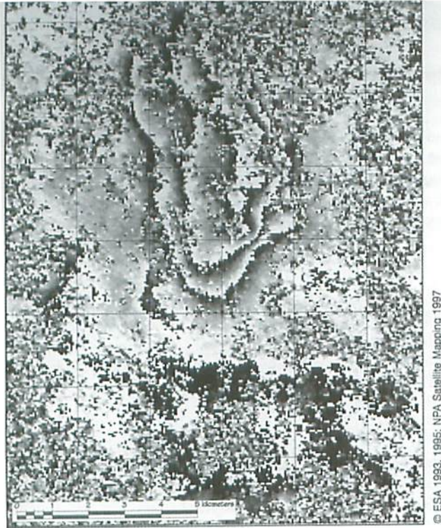
a. An interferogram covering an urban area 12 km x 16 km in size, made with ERS images taken 2 years 4 months apart
