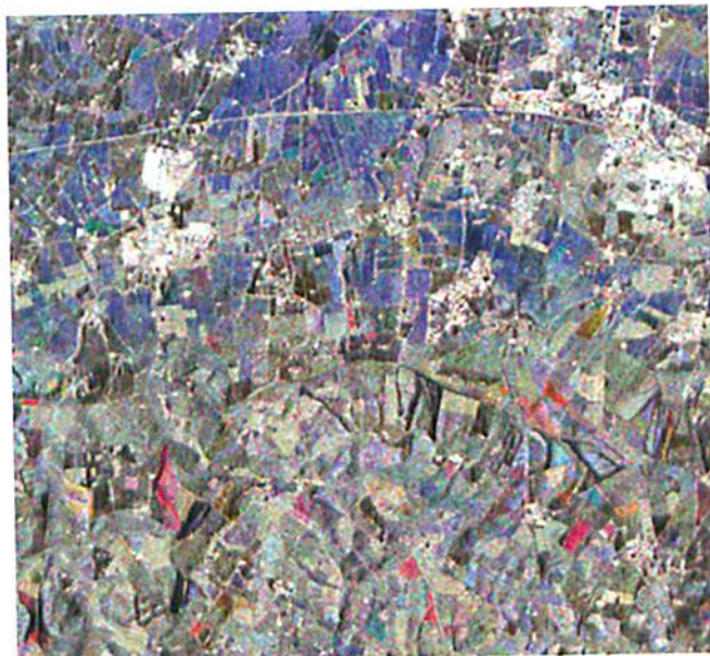
Figure 4.5 Multi-incidence angle composite for Thames, UK, produced from 3 Radarsat images (Blue: 23° 23 March 97, Green: 37° 13 March 97, Red: 43° 3 March 97) (Acknowledgment: Remote Sensing Applications Consultants, Alton, UK & Radarsat Data Copyright Canadian Space Agency/Agence spatiale canadienne 1997).
