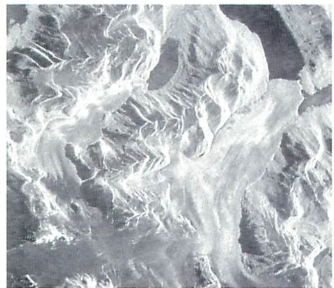
Figure 5.8 ERS and Radarsat images of the Moreno and Ameghino Glacier, Southern Patagonia, Argentina. These show differences in terrain distortion between the top image (ERS) acquired with an incidence angle of 23° and the bottom image (Radarsat) ( incidence angle of 47°). (Acknowledgment: H.Rott, Institut für Meteorologie und Geophysik, Innsbruck, Austria).
