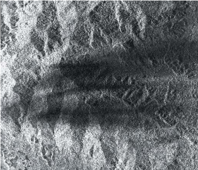
Figure 17: The effect of rain clouds can be seen as a darkening on the image in the region where the radar signal strength was reduced.
