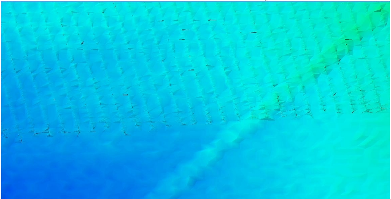
Figure 2: Profile of the surface generated by combining LIDAR data from flight lines 1 and 2. Note how it is noisier than either of the surfaces 1 and 2 as it is influenced by them both.
