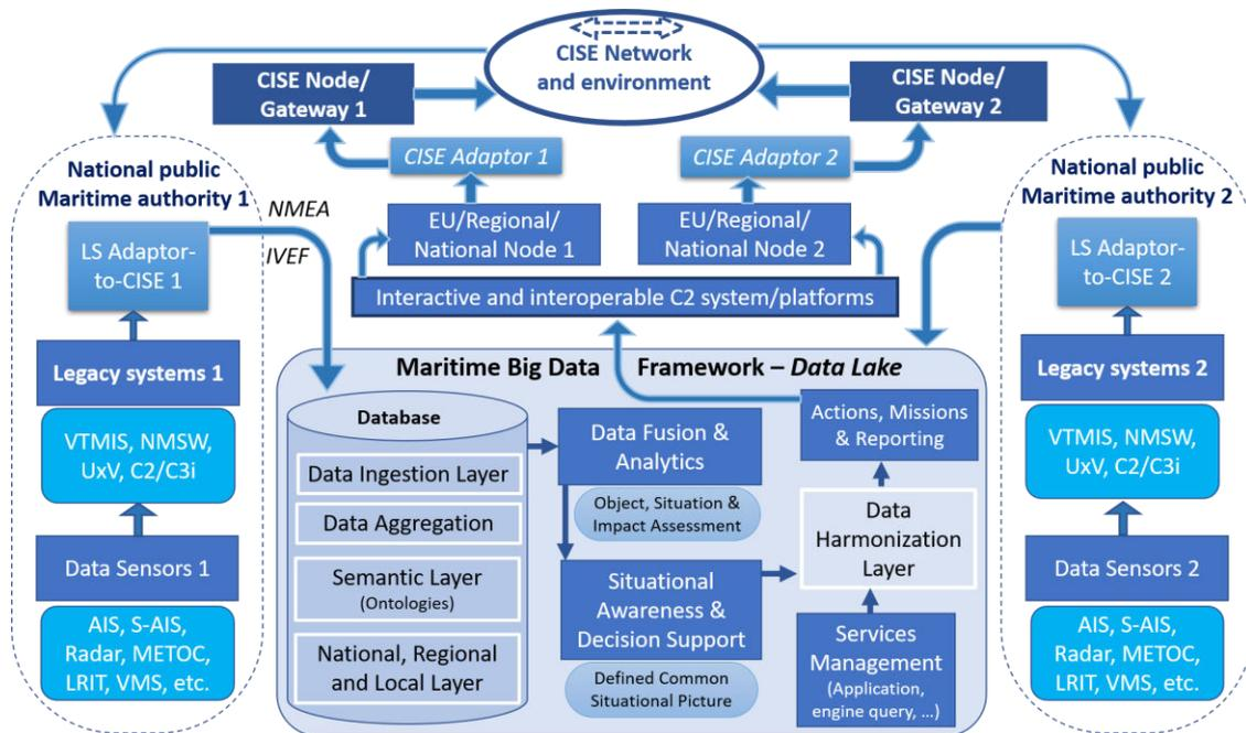
Figure 1. General CISE Hybrid Architecture with integrated Maritime Big Data Framework (authors adapted according to the [6],[7],[8])
