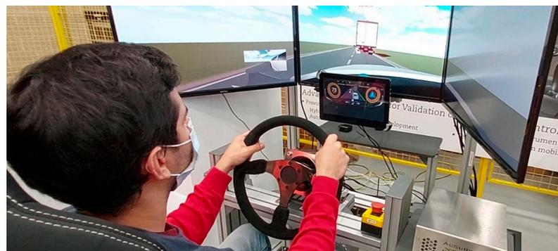
**Figure 2.** DiL simulator for AD applications with Dynacar vehicle simulation software in screens, and Re:Lab HMI as the instrument cluster.
