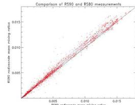
Figure 6. RS90 mass mixing ratio versus RS80 mass mixing ratio. Good agreement is seen at all mixing ratios although the RS90 has a slight wet bias.
