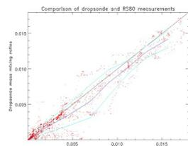
Figure 8. Dropsonde mass mixing ratio versus RS80 mass mixing ratio. A dry bias can be seen at all mixing ratios, becoming significant at high mixing ratios.
