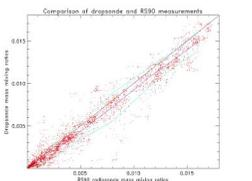
Figure 11. RS90 dropsonde mass mixing ratio versus balloon-borne RS90 mass mixing ratio. The two instruments, which have the same type of sensor element agree to within one standard deviation although a dry bias is evident in the dropsonde data.
