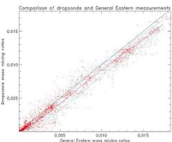
Figure 2. Dropsonde mass mixing ratio versus General Eastern mass mixing ratio. A dry bias of about 1.0% is seen in the dropsonde mixing ratios above 11 g/kg.
