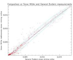
Figure 4. Snow White mass mixing ratio versus General Eastern mass mixing ratio. Good agreement between these instruments.
