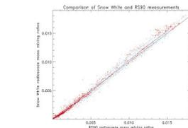
Figure 12. Snow White mass mixing ratio versus RS90 mass mixing ratio. Reasonable agreement is seen at all relevant mixing ratios a possible wet bias in the Snow White data is evident at higher mixing ratios. All Snow White sondes were flown in tandem with RS90s.
