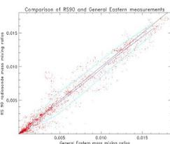
Figure 3. RS90 mass mixing ratio versus General Eastern mass mixing ratio. Good agreement between these instruments is seen throughout the range of mixing ratios encountered although there is some suggestion of a dry bias in the RS90 at high mixing ratios.
