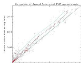
Figure 10. General Eastern mass mixing ratio versus RS80 mass mixing ratio. A wet dry bias in the General Eastern becomes evident at mixing ratios above 6 g/kg.
