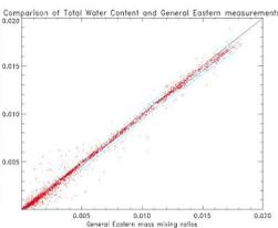
Figure 1. Total water content mass mixing ratio versus General Eastern mass mixing ratio. A slight, but not significant, dry bias is seen in the total water probe.
