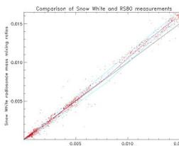
Figure 7. Snow White mass mixing ratio versus RS80 mass mixing ratio. Although good agreement is seen in dry conditions the Snow White exhibits a significant wet bias at high mixing ratios.
