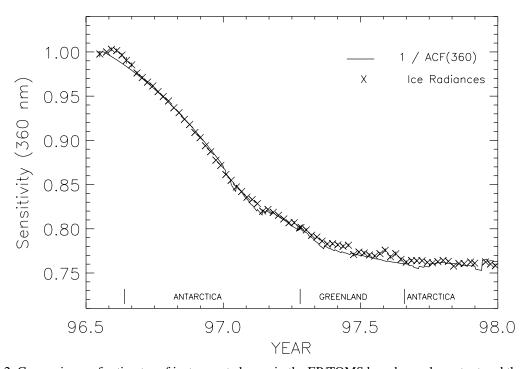
Figure 3.2. Comparisons of estimates of instrument change in the EP/TOMS based on solar output and the reflectivity of Antarctica and Greenland.
