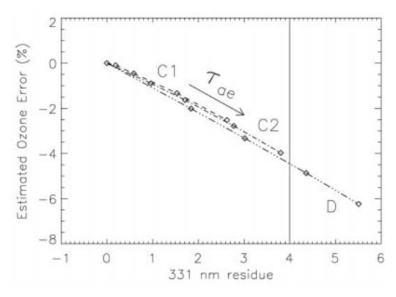
Figure 6.1. TOMS Derived Ozone Error as a Function of Aerosol Index in the Presence of Tropospheric Absorbing Aerosol. (D) Desert dust (C1 and C2) Smoke.
