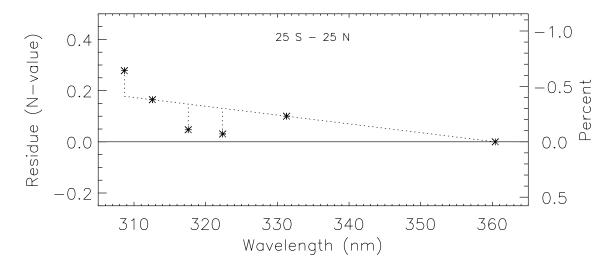
Figure 4.1. Modes of Equatorial Distributions of Residues for Each of the EP TOMS Channels as a Function of Wavelength. Residues are reported on the Level-2 product in units of N-value. A difference of 1 N-value is equal to 2.31%.
