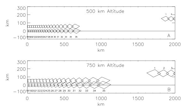
Figure 2.1 Earth Probe TOMS Instantaneous Fields of View Projected onto Earth's Surface. The right portion (samples 18-35) of two consecutive scans are shown, and a portion of a scan from the previous orbit is also shown to illustrate the degree of inter-orbit coverage at the equator for: a) 500 km orbit altitude, and b) 750 km orbit altitude. The higher orbit after December 1997, results in 90% daily global coverage (84% at equator and 100% at 30° latitude).
