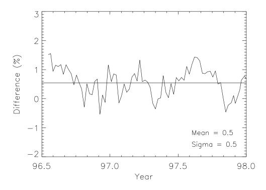
Figure 5.3. Percentage Difference of TOMS - ground ozone measurements as a function of time.
