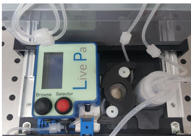
Figure 7. LivePa is connected to a LiveBox1 and the IVTech fluidic circuit to mimic the environmental conditions of glaucoma
