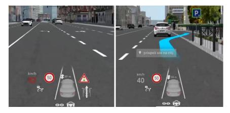
Figure 1. Left: Visual 2D HUD (MAX version); Right: Visual AR HUD (MIN version)
