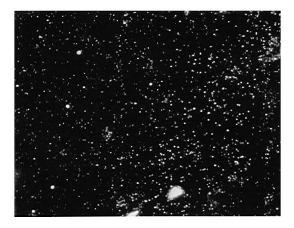
FIG. 1: Hidden domains in water exposed to halogen light for 37.5 hours, revealed by a novel microscope technique using side illumination. These are 0.2 to 1.5 microns in size, with a few exceptions.
