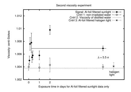
FIG. 7: Repeat of the viscosity experiment to determine the effect of aluminium-foil filtered sunlight on distilled water. The sun only lasted two days and so the number of data points is limited. The average of the right-hand five data points exceeds that of the three controls by 5.6  $\sigma$ , 8.4  $\sigma$ , and 4.0  $\sigma$  respectively. These results confirm the previous experiment and show that the effect is reproducible.
