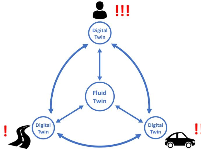
**Fig. 3.** Fluid digital twins. Driver (top), vehicle (right) and environment (left) models, as well as their possible interactions, are represented and updated inside the central fluid digital twin with different priority, as indicated by the number of exclamation marks.
