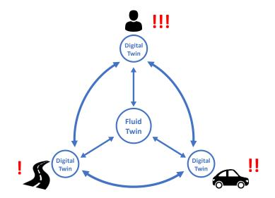
**Fig. 3.** Fluid digital twins. Driver (top), vehicle (right) and environment (left) models, as well as their possible interactions, are represented and updated inside the central fluid digital twin with different priority, as indicated by the number of exclamation marks.
