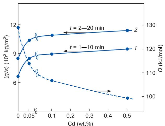
**Figure 4.** Isochrones of oxidation (723 K) of the aluminum conductive alloy E-AlMgSi (Aldrey) doped with cadmium
