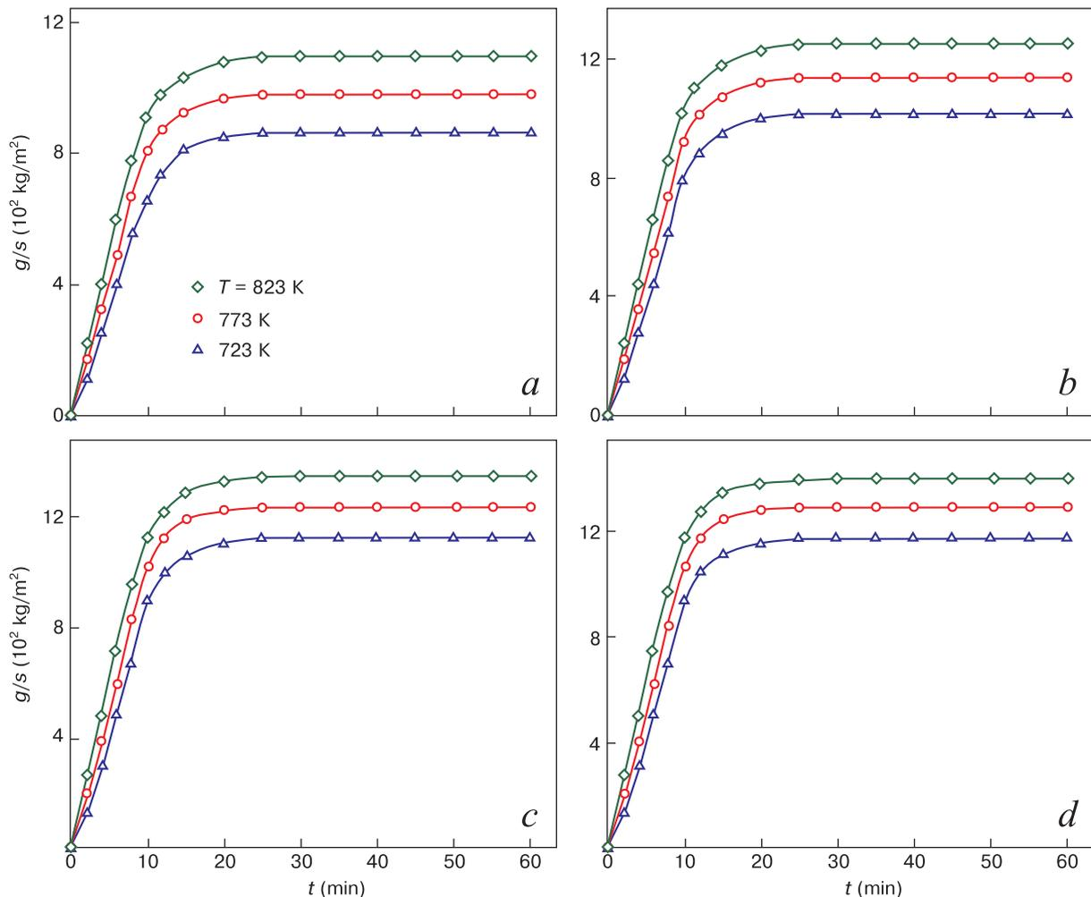
**Figure 1.** Kinetic curves of oxidation of the aluminum conductive alloy E-AlMgSi (Aldrey) (a) doped with cadmium, wt.%: 0.05 (b); 0.1 (c); 0.5 (d)
