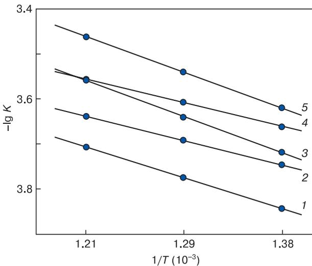
**Figure 3.** Dependence of  $\lg K$  on  $1/T$  for aluminum conductive alloy E-AlMgSi (Aldrey) (1) doped with cadmium (wt.%): 0.01 (2), 0.05 (3), 0.1 (4), 0.5 (5)
