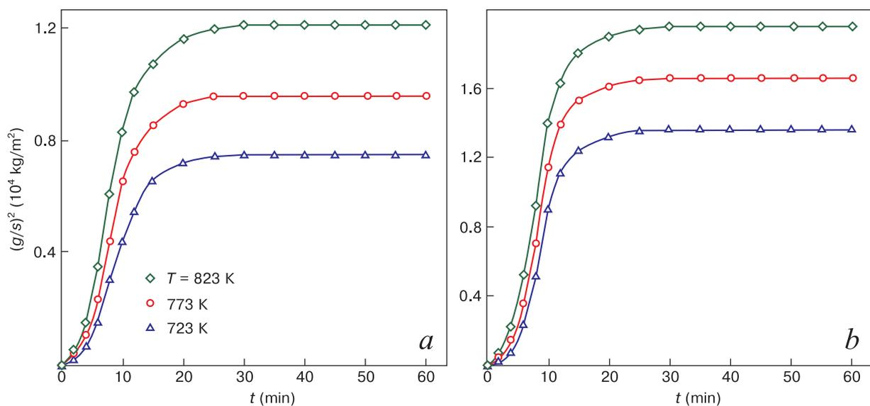
**Figure 2.** Quadratic kinetic curves of oxidation of an aluminum conductive alloy E-AlMgSi (Aldrey) (a) doped with 0.5 wt.% cadmium (b)
