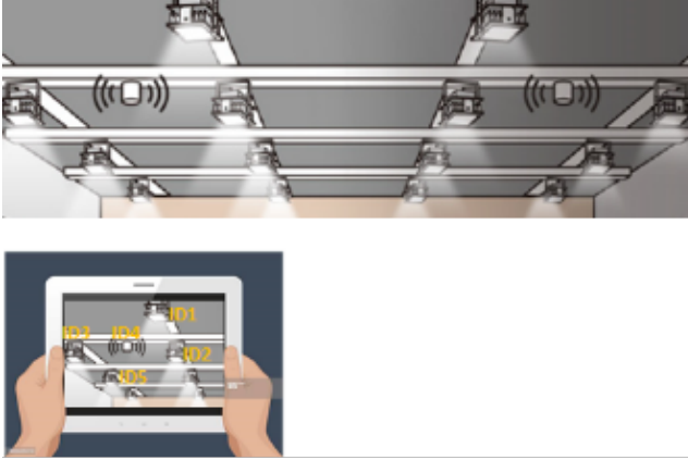
Figure 1: LiTalk: VLC-based collection & mapping of light IDs.
