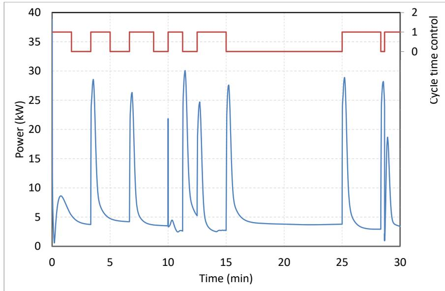
Figure 6: Adsorption machine output power (adsorption/desorption cycle control as a function of the temperature)- The red line indicates the feedback signal based on  $T_{\text{user,measured}} - T_{\text{user,set}}$
