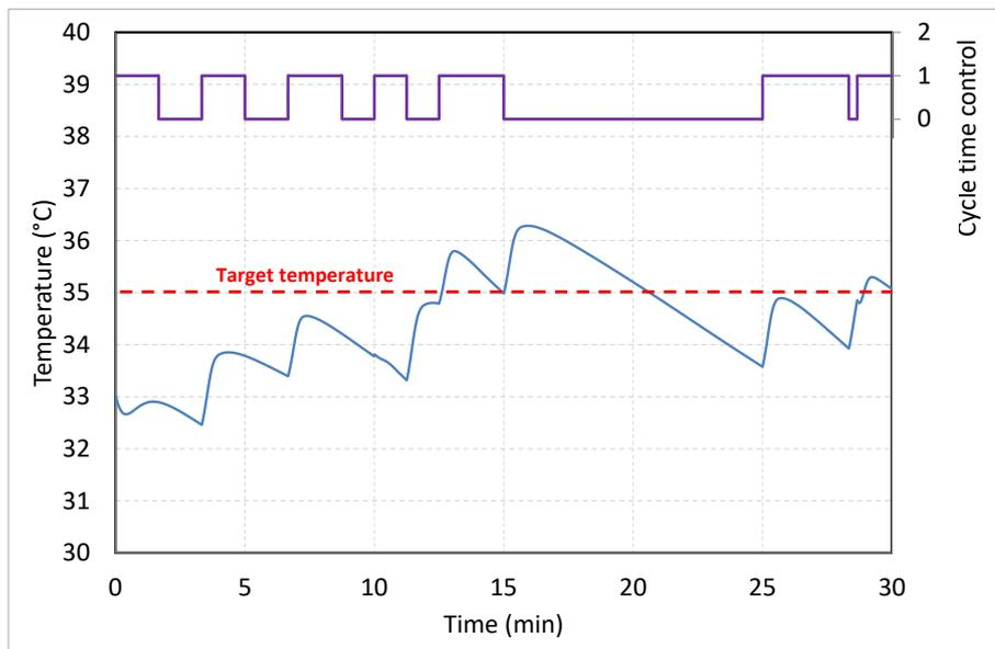
Figure 7: Temperature of the water delivered to the user using the feedback control
