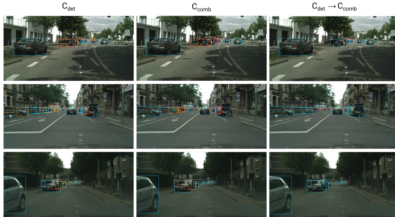
Figure 3. Qualitative results on Sim10K \rightarrow Cityscapes scenario of ConfMix models trained with different confidence settings. We visualise true positives in blue bbx, false negatives in red bbx and false positives in orange bbx. By introducing a gradual transition between confidence metrics, we achieve less false positive detections compared to training only using C_{det} and less false negative detections compared to training only using C_{comb} .
