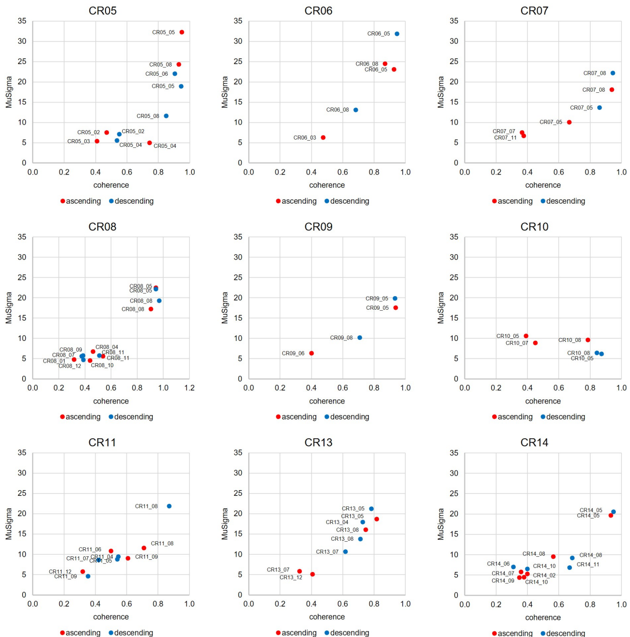
Figure 5. The MuSigma and coherence values for the pixels representing the corner reflectors and their closest surroundings in LoS slant geometry issued from SARscape routine both for ASC and DESC orbits
