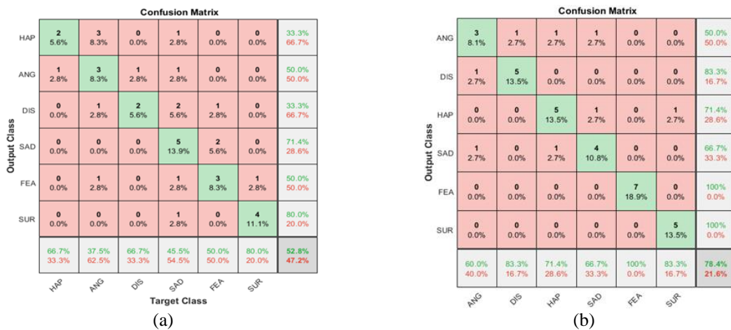
Figure 8. The testing confusion matrix using kNN classifier for JAFFE dataset using, (a) HOG feature set and (b) LBP feature set
