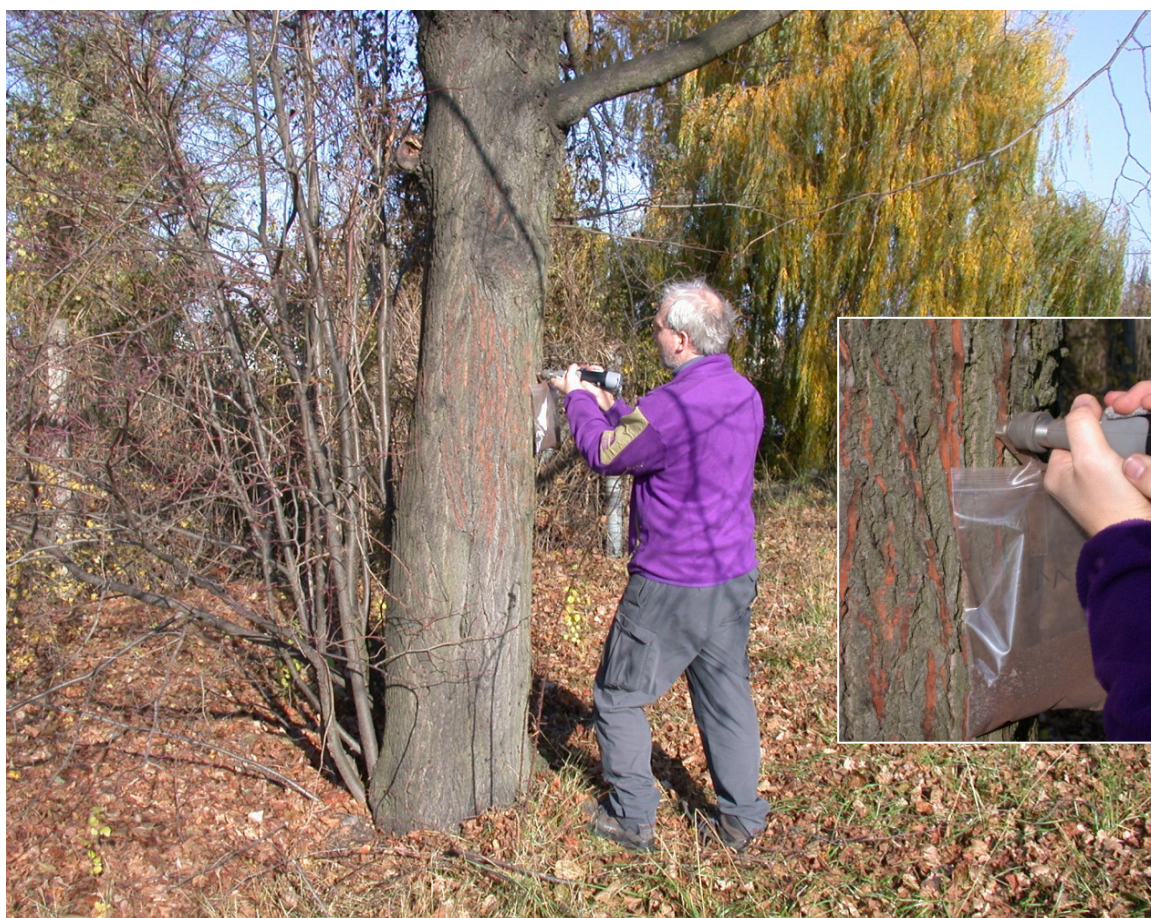
Photo 17. Sampling of outer bark at location S11 (Industrial Street) in the Stassfurt urban area, Germany (high speed milling cutter with a special titanium nitrite bit, sampling depth: 1 mm, milling speed 15,000 rpm (Source: Birke et al. , 2009, Fig. 200, p.327).
