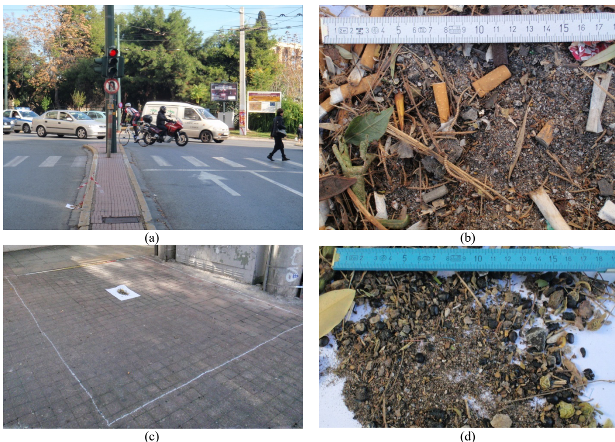
Photo 15. Road dust or road sediment sampling from a junction: (a) road junction near the Temple of Olympian Zeus, Athens, Hellas – the sample was collected from the left gutter, and the road dust sample has been placed on a white piece of paper and is marked by wooden stick with red-white ribbon; (b) close-up of road dust, which is a heterogeneous mixture of dust particles, plant remains, cigarette (bad habit of Hellene drivers to throw the butt-ends of their cigarettes on the road); (c) sampling of road dust from the pavement at the road junction – the pavement within the marked area was swept and pavement dust is on the white sheet of paper; (d) close-up of the road pavement dust, which is again a heterogeneous mixture of dust particles, small stones and plant remains (Source: Demetriades, 2014, Photo 15, p.25).
